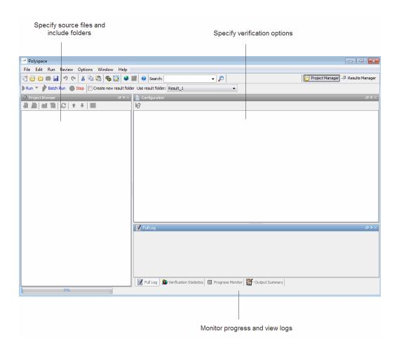
By default, the Polyspace verification environment displays the Project Manager perspective. The Project Manager perspective has three main sections.
