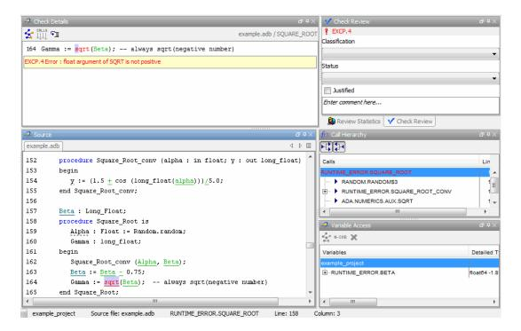
You see the section of source code where this error occurs, and details about the check in the **Check Details** pane..
