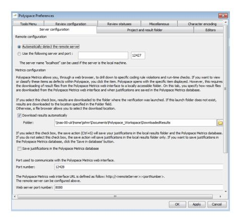
By default, Polyspace software automatically finds the server. You can specify the server by selecting **Use the following server and port** and providing the server name and port. For information about setting up a server, see the *Polyspace Installation Guide*.
