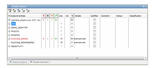
The package RUNTIME\_ERROR is red because it has run-time errors. Polyspace software assigns each package the color of the most severe error found in the package. The first column of the Procedural entities view contains the name of the procedural entity (package or function). The following table describes some of the other columns in the procedural entities view.
