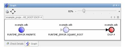
The code associated with  ${\tt EXCP.4}$  is in  ${\tt SQUARE\_ROOT}.$  The function <code>MAINRTE</code> calls  ${\tt SQUARE\_ROOT}.$
