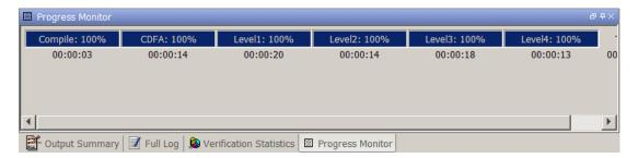
The progress bar highlights the current phase in blue and displays the amount of time and completion percentage for that phase.
