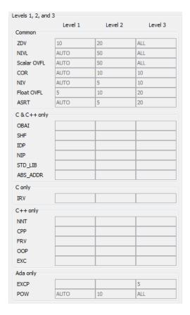
For example, when you select level 1, the table specifies that you review ten orange ZDV checks. The number of checks increases as you move from level 1 to level 3, reflecting the changing review requirements as you move through the development process.
